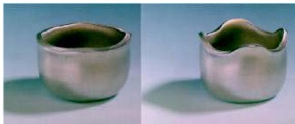
**Figure 1** – ‘Earing’ of a cup after deep-drawing from a rolled sheet of aluminium (source <http://aluminium.matter.org.uk>)
