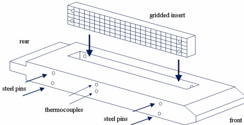
**Figure 2** – View of the specimen and gridded insert.
