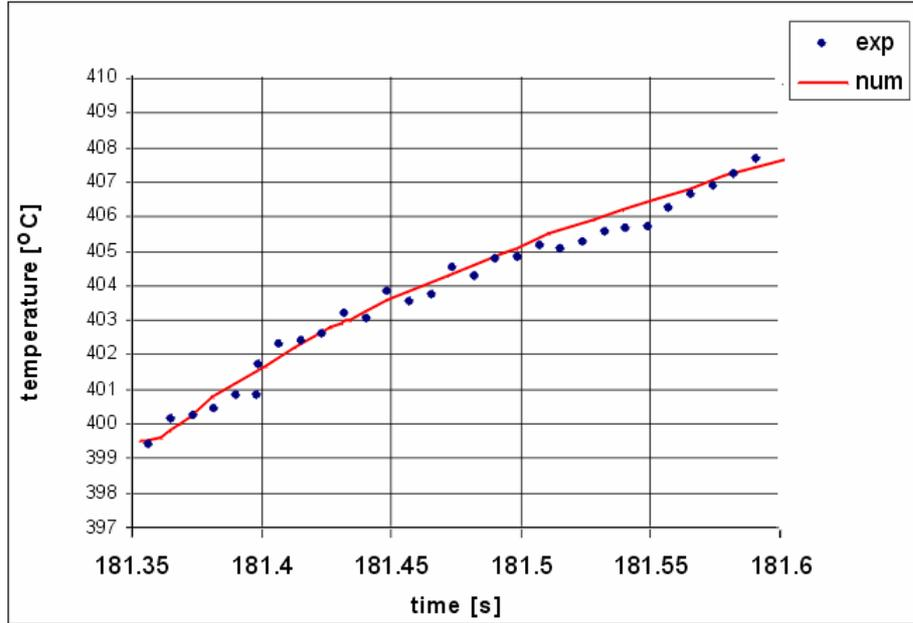
**Figure 8** – Experimental and numerical temperatures extracted from the sample and from the 2D FE model
